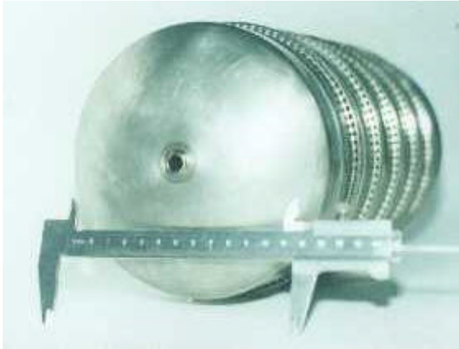
Fig 8. The cell for solid deuterium source.
