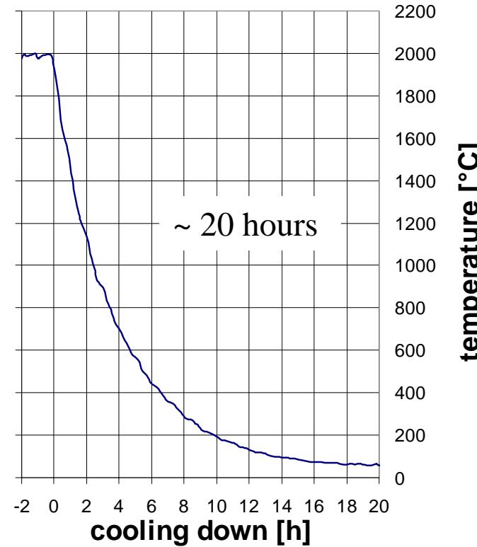
measured by the noise thermometer - reactor power 20 MW
