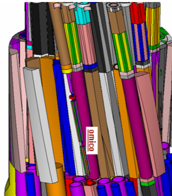
Fig.4 Position of the OMICO fuel bundles grouping of 8 MOX fuel rods each
