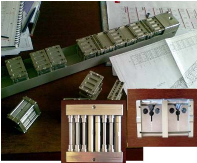
Fig. 7 : up : Tray containing baskets down : tensile and fracture toughness baskets
