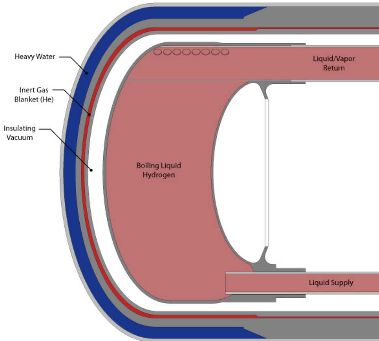
Figure 3. Cross section of the BT-9 cold source moderator vessel (nearly to scale; the  $\text{LH}_2$  ID is 11 cm). The source is surrounded by insulating vacuum, a He containment, and a  $\text{D}_2\text{O}$  cooling jacket. At the top is a piccolo-like phase separator at the inlet of the vapor return line, to ensure the vessel is filled.
