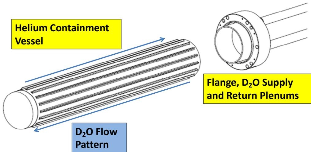
Figure 6. A portion of the assembly drawing of the He containment vessel and the flange that mates with the surrounding D<sub>2</sub>O jacket.
