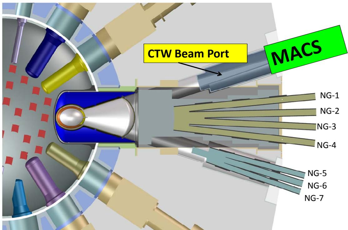
Figure 2. Existing cold source and neutron guides. The new guides will be installed in CTW, and MACS will be relocated to BT-9 (not shown), and have its own cold source.
