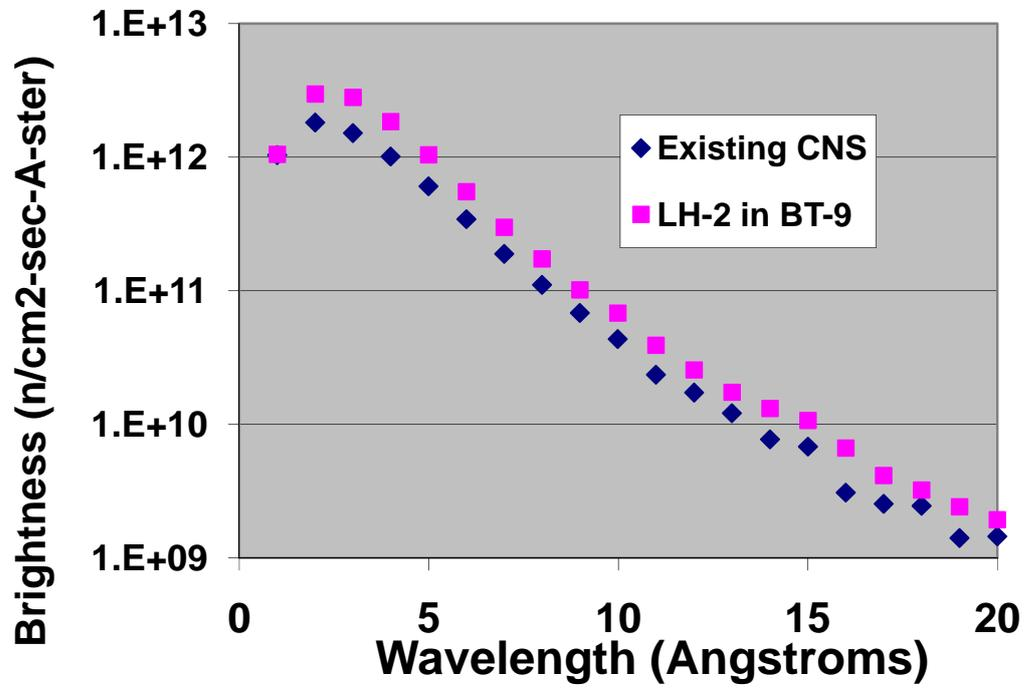
Figure 4. Brightness of the BT-9 source and the existing Unit 2 CNS. The intensity gain varies from 1.7 to 2.
