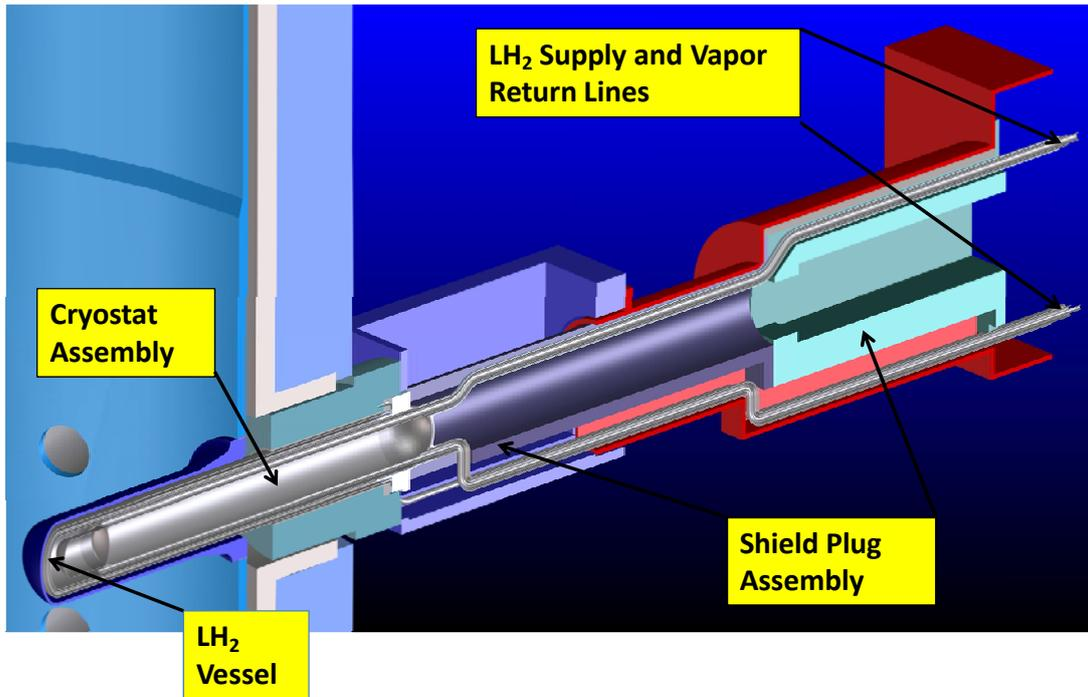
Figure 5. Cut-away view of the cryostat and shield plug assemblies to be inserted horizontally into BT-9.
