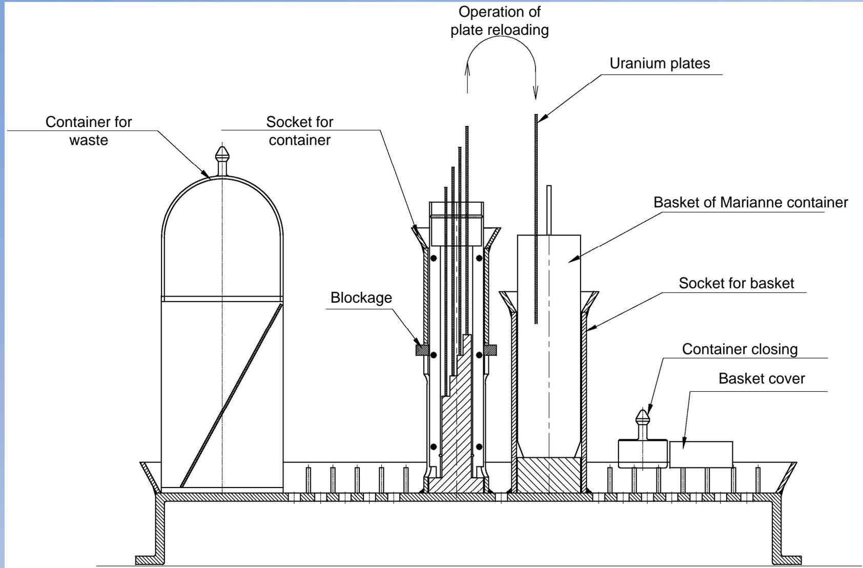
*Fig.12. Scheme of irradiated plates reloading inside the hot cell*
