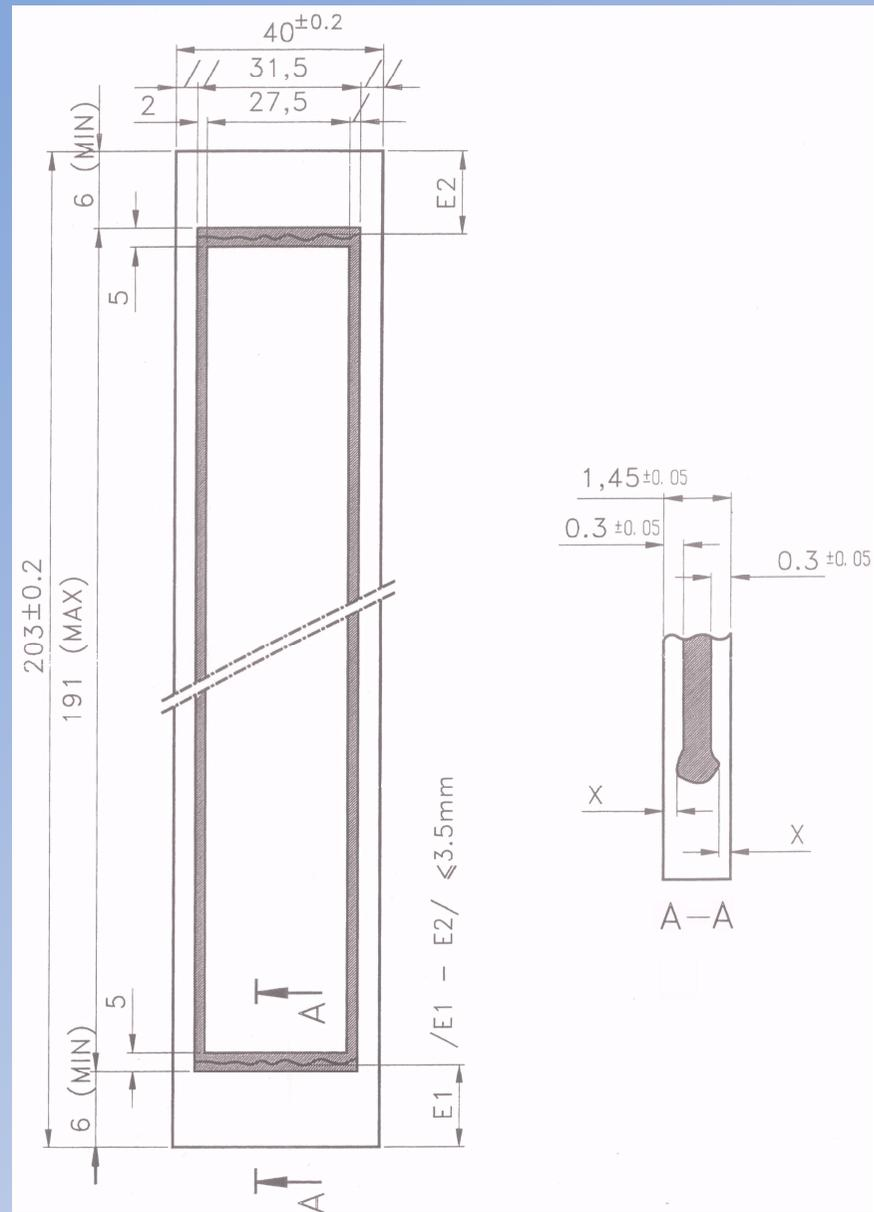
**Fig.6. Uranium plate containing HEU (93% U<sup>235</sup>)**
