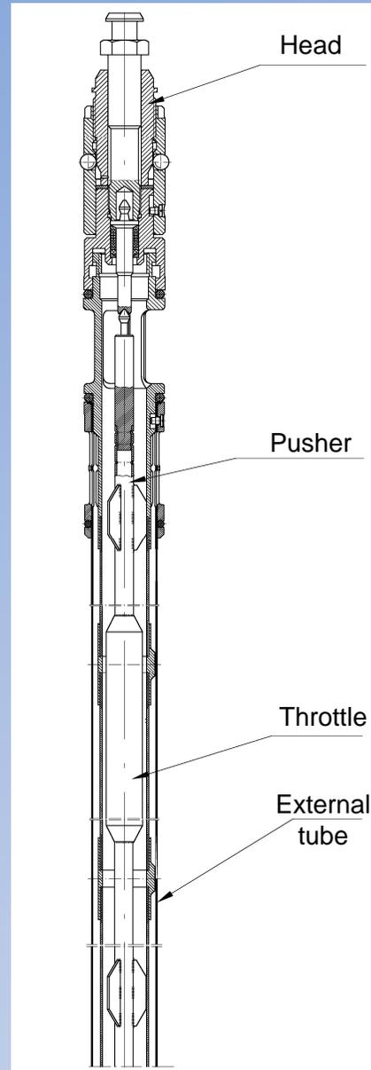
*Fig.8. Upper part of irradiation channel*
