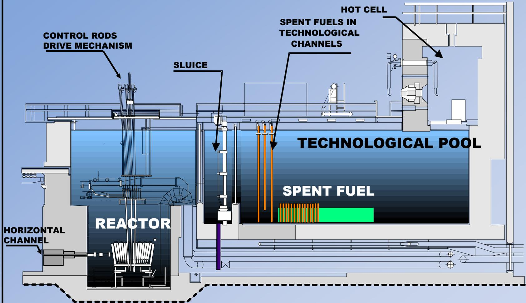
*Fig.3. Cross section of the reactor pools*
