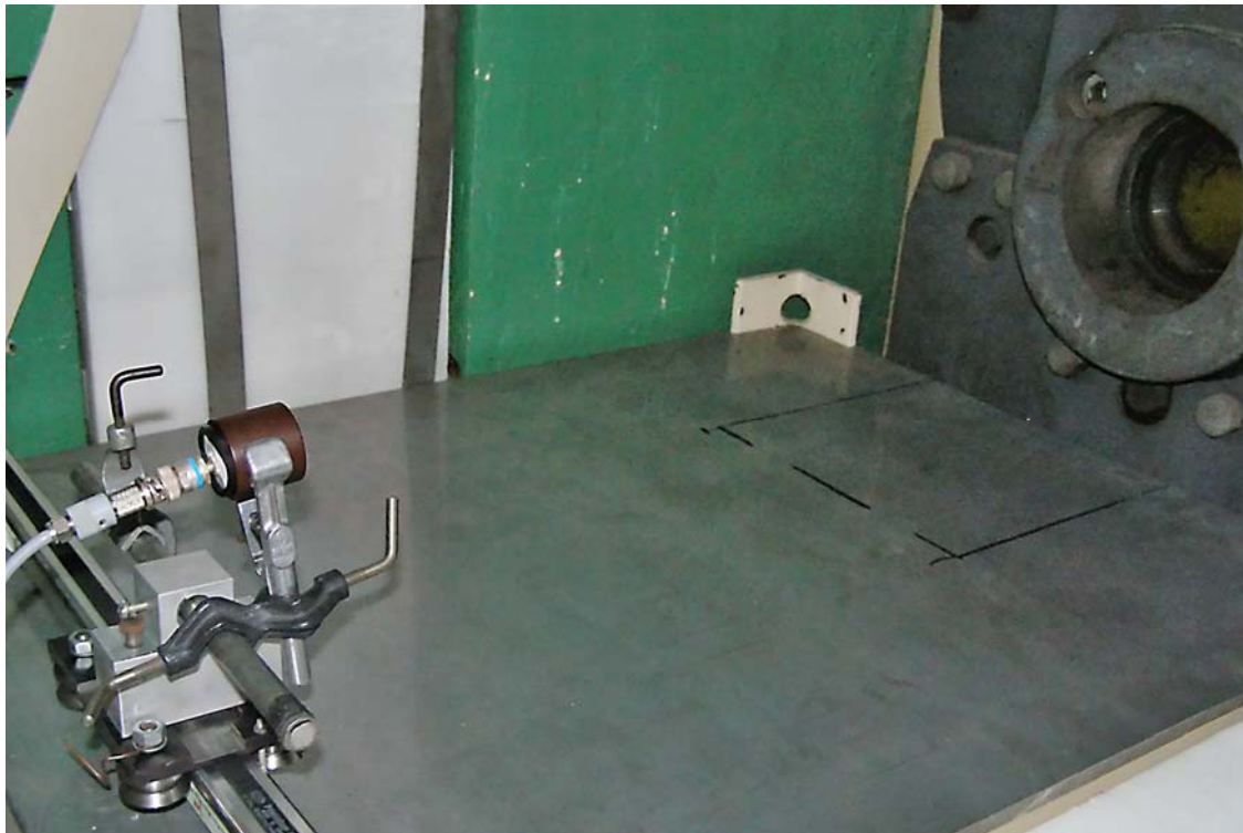
Fig. 2. Measurement of spatial distribution of the thermal neutron beam, left – detector with the positioning device; right – beam outlet
