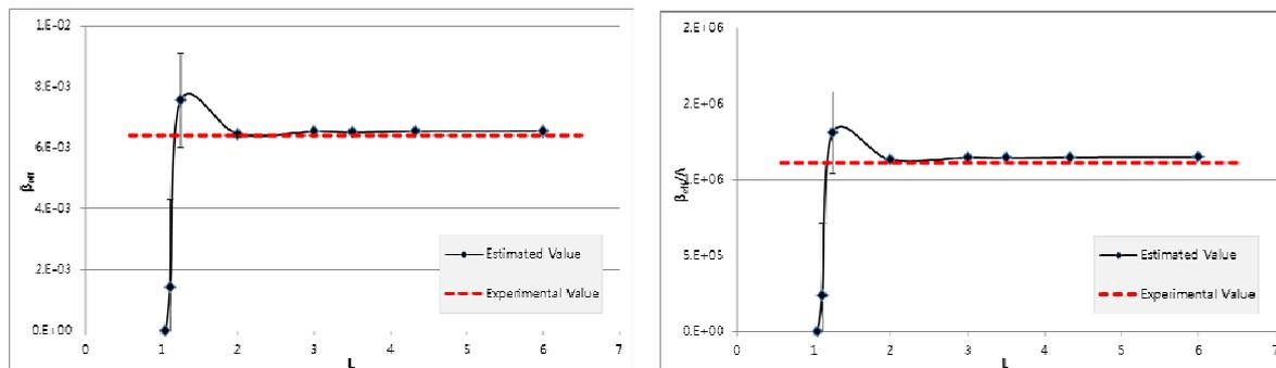
**Figure III. Comparisons of adjoint-weighted kinetics parameters in the MC Wielandt calculations for Godiva problem with varying  $L$**
