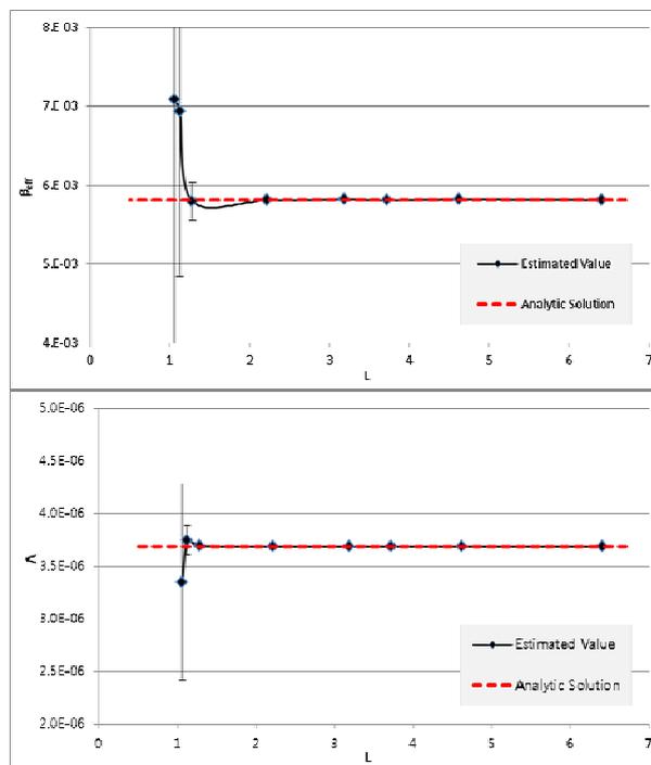
**Figure I. Comparisons of adjoint-weighted kinetics parameters in the MC Wielandt calculations for the infinite homogeneous problems with varying  $L$**
