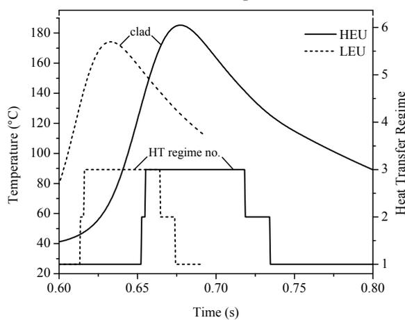
FIG. 10. Heat transfer regime and clad temperatures during FRIA
