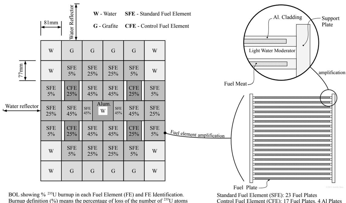
FIG. 6. Core and fuel elements schematic for the IAEA benchmark problem
