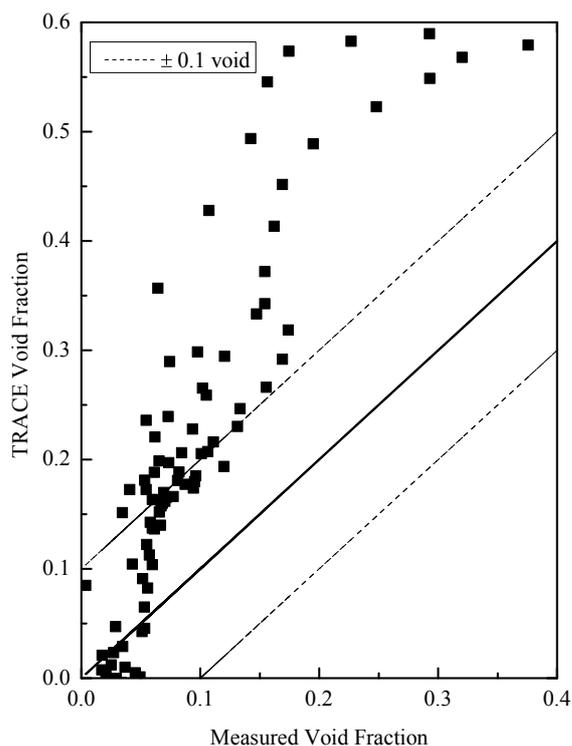
FIG. 4 Void fraction measurements vs. TRACE predictions
