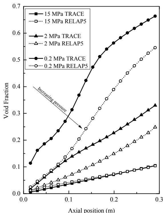
FIG. 5. RELAP5 vs. TRACE void fraction predictions at various pressures
