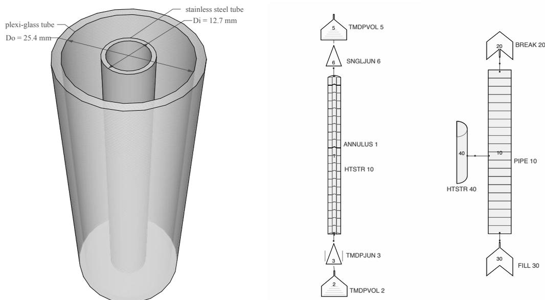
FIG. 1. Sketch of the heated section (left), and nodalizations for RELAP5 (center) and TRACE (right)
