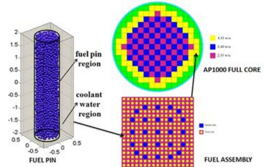
FCM fueled LWR configuration at different dimensional levels: from TRISO fuel particle to LWR core assembly
