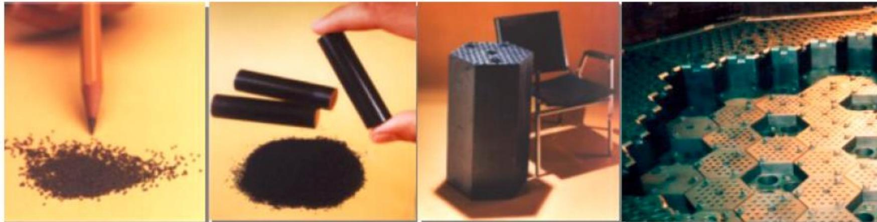
**Prismatic-block gas-cooled reactor fuel configuration. From left to right: TRISO fuel particle, fuel compact, fuel block, and reactor core.**
