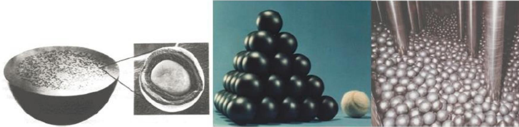
**Pebble-bed reactor fuel configuration. From left to right: TRISO fuel particle, fuel pebbles, and reactor core.**
