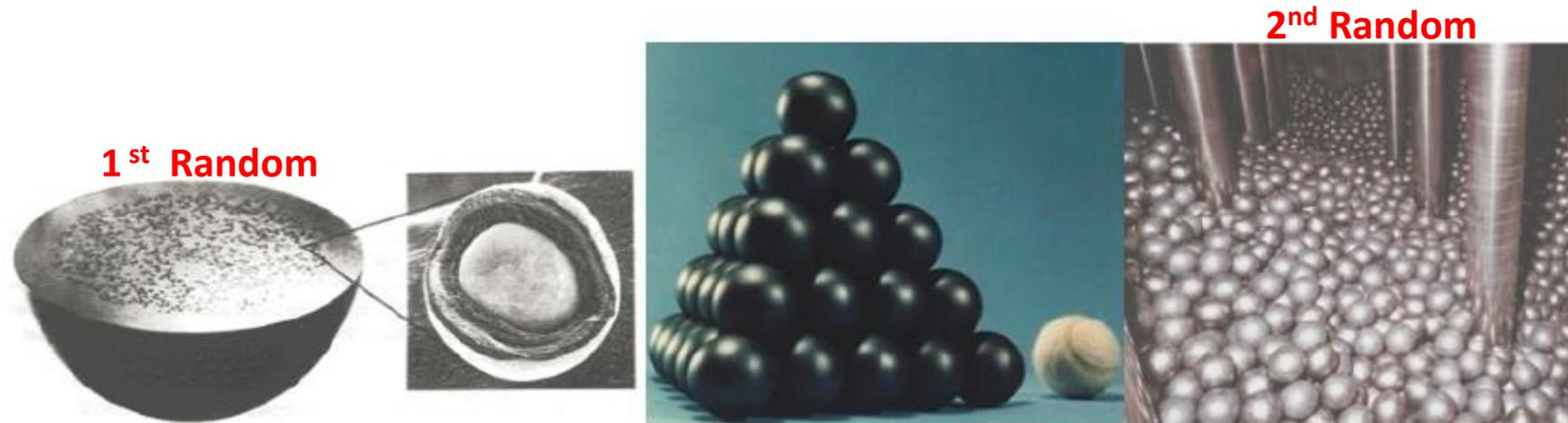
**Pebble-bed reactor fuel configuration. From left to right: TRISO fuel particle, fuel pebbles, and reactor core.**
