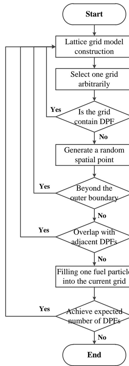
The basic principle and implementation procedure of the SFL method.
