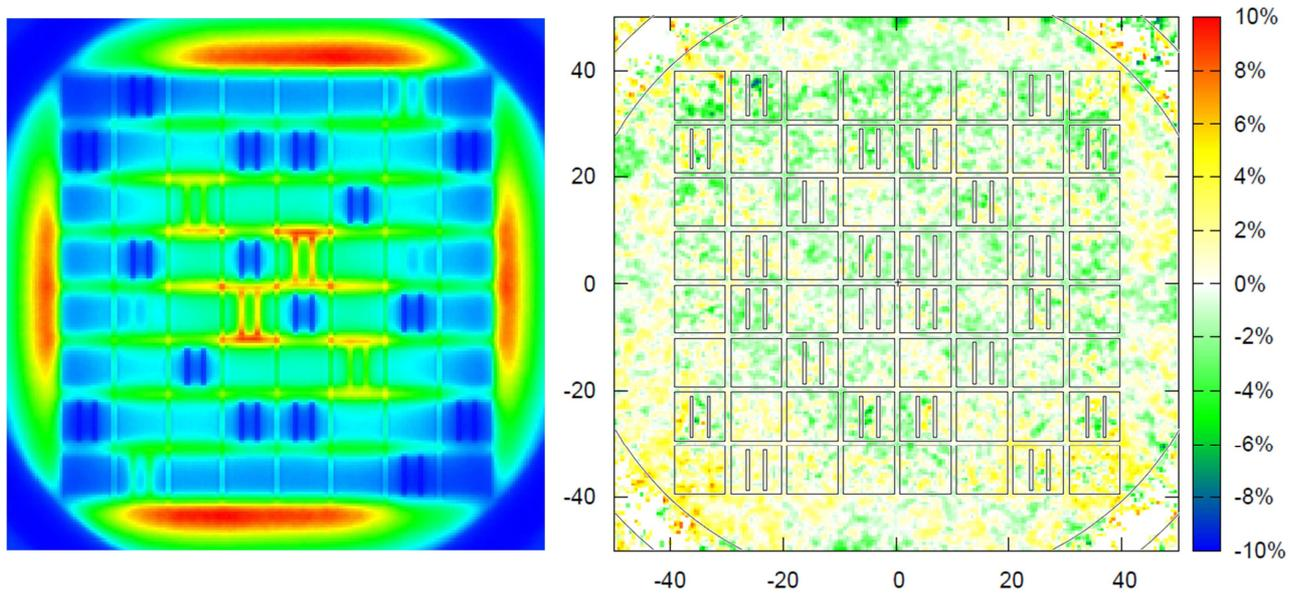
FIG. 7: Thermal flux in the critical state (TRIPOLI4©, left) and comparison MCNP6 vs. TRIPOLI4© (% , right)
