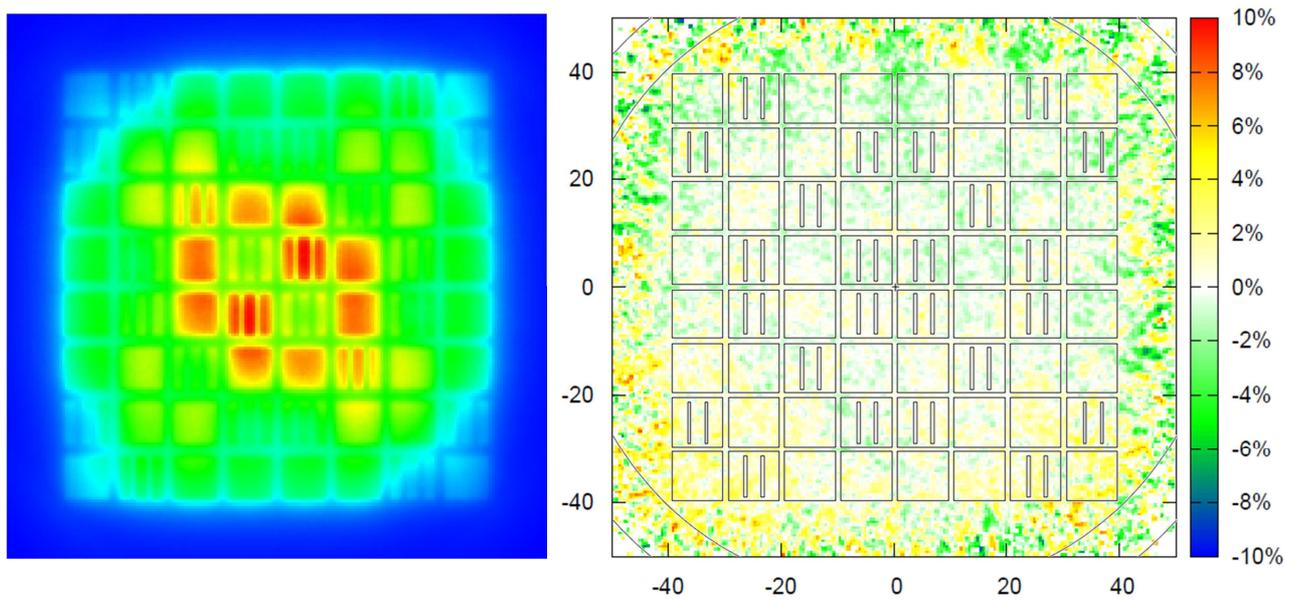
FIG. 9: Fast flux in the critical state (TRIPOLI4©, left) and comparison MCNP6 vs. TRIPOLI4© (%), right)
