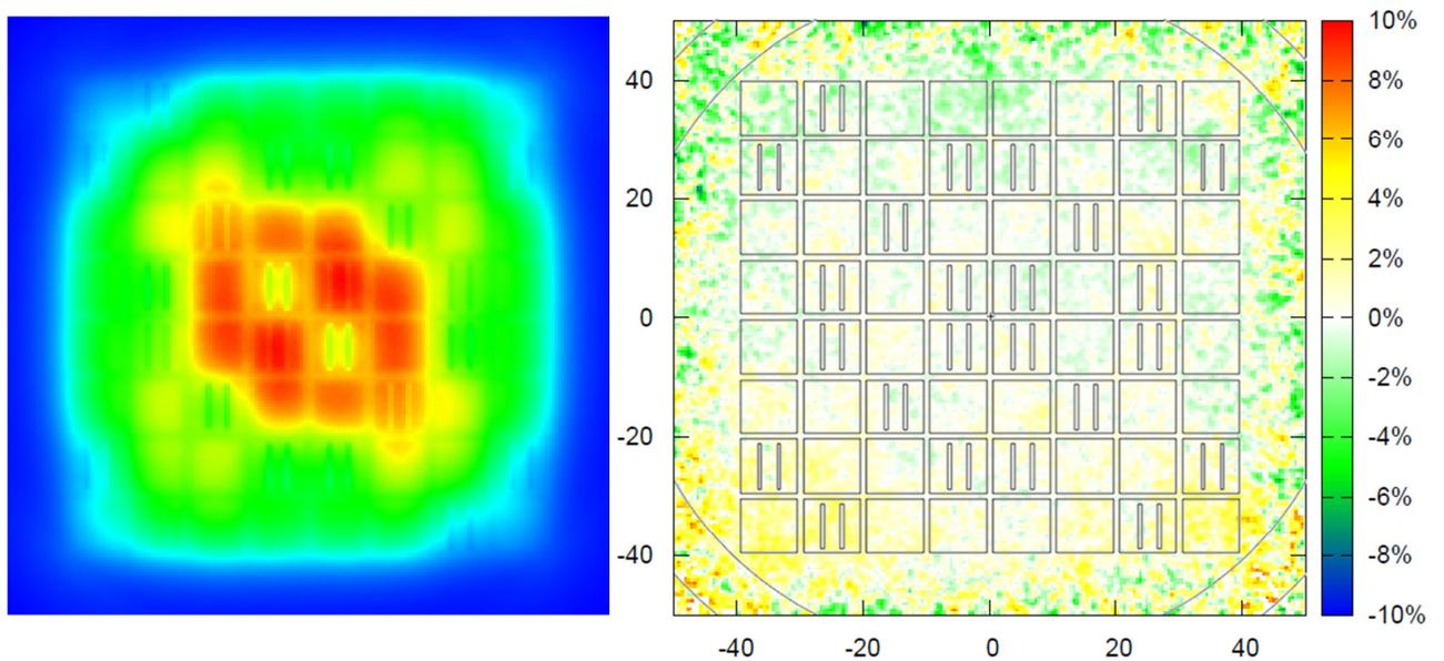
FIG. 8: Epithermal flux in the critical state (TRIPOLI4©, left) and comparison MCNP6 vs. TRIPOLI4© (% , right)
