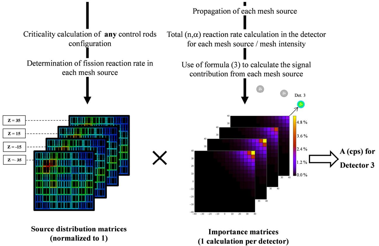
FIG. 12. Detector response calculation with Green Functions
