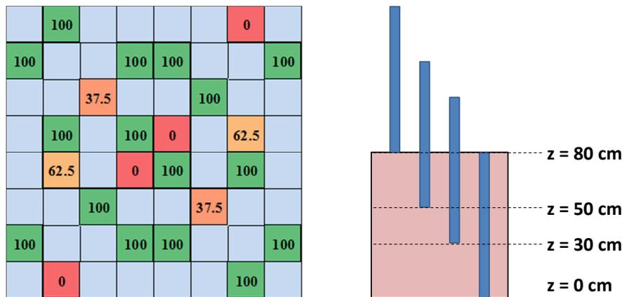
FIG. 6. Insertion percentage and corresponding altitude of each control rod leading to a critical state
