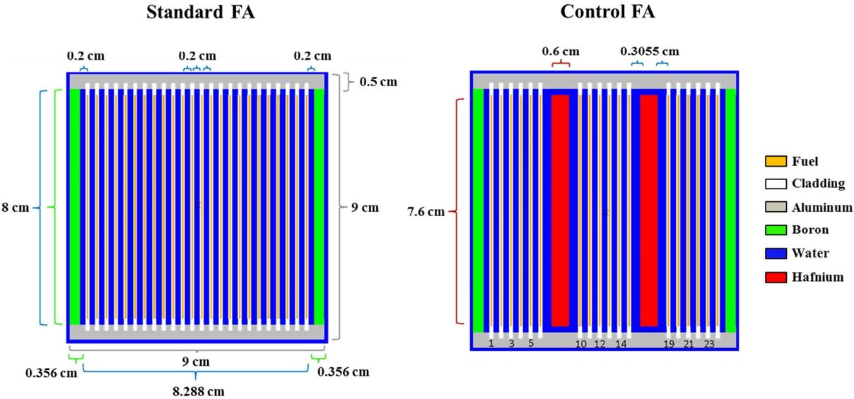
FIG. 2. Cross section geometry for both standard (left) and control assemblies (right)
