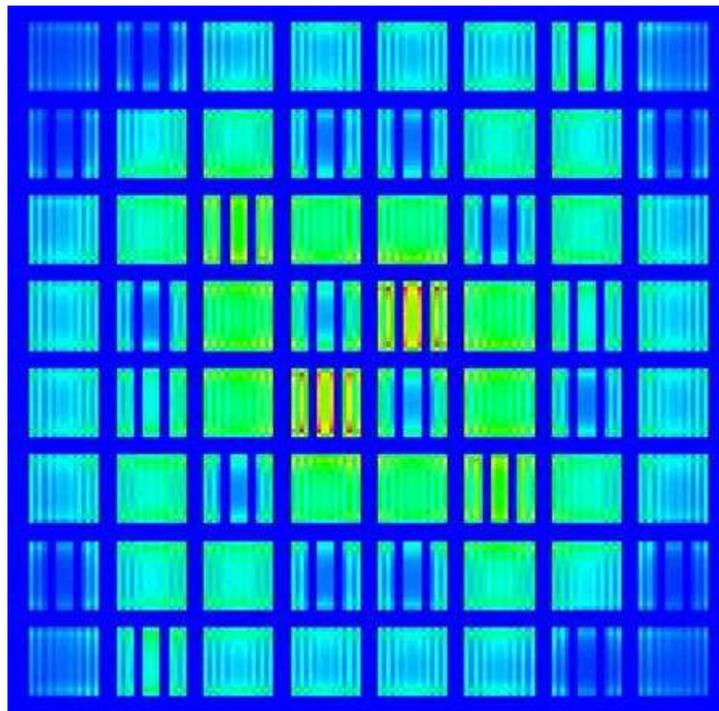
FIG. 10: Fission power distribution in the critical state (TRIPOLI4©)
