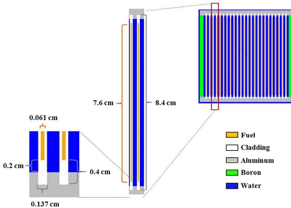
FIG. 1. Cladding and fuel geometry (fuel plate and assembly)
