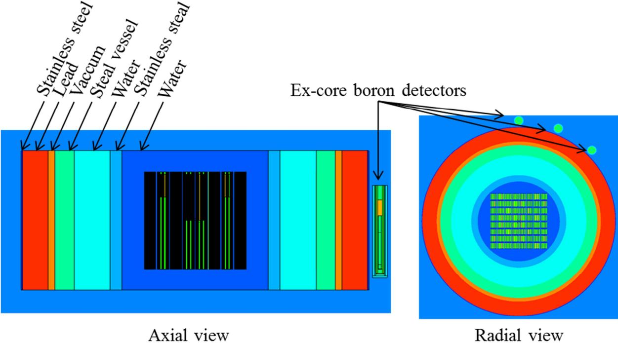
FIG. 5. Vertical and horizontal cross sections of the core in its environment
