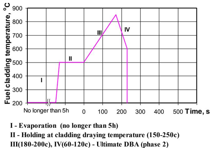
FIG.5. Temperature scenario of the LOCA simulation experiment.
