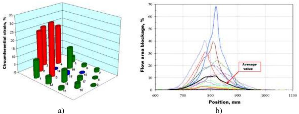
FIG. 10. Maximum circumferential strain of claddings in the test fuel assembly (a). Changes in the cross-sectional flow area of the coolant (b).
