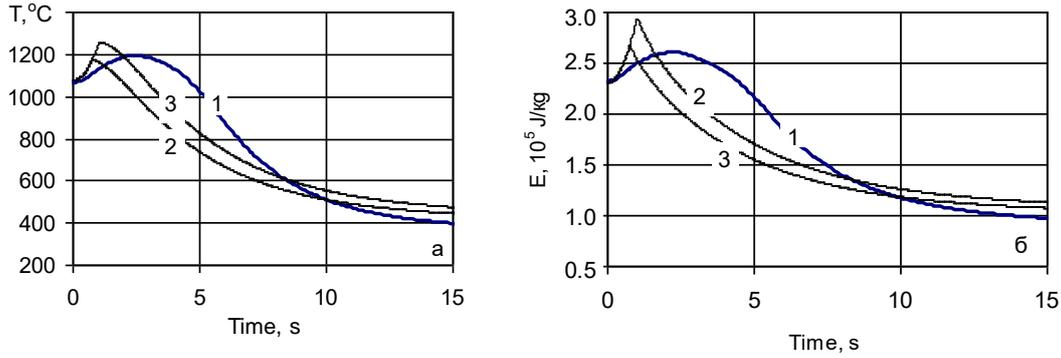
FIG. 2. Changes in the temperature in the center of fuel stack for irradiated fuel rodlet (a) and radial average enthalpy (b) of irradiated fuel as a function of time at different parameters of pulse: 1- calculated profiles for the VVER-1000 fuel; 2-3 – calculated profiles for pulse irradiation tests in the MIR reactor at a linear heat generation rate of 250 W/cm (initial value), pulse amplitude of 3.25,  $\tau=0$ (2);  $\tau=0.5$ s(3).
