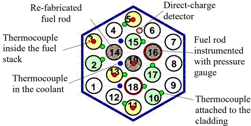
FIG. 4. Schematic arrangement of fuel rodlets, thermocouples and sensors in the test assembly.
