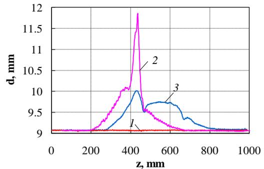
FIG. 15. Profile diagrams of the cladding and fuel rodlets before (1) and after test #1 (2) and #2(3).
