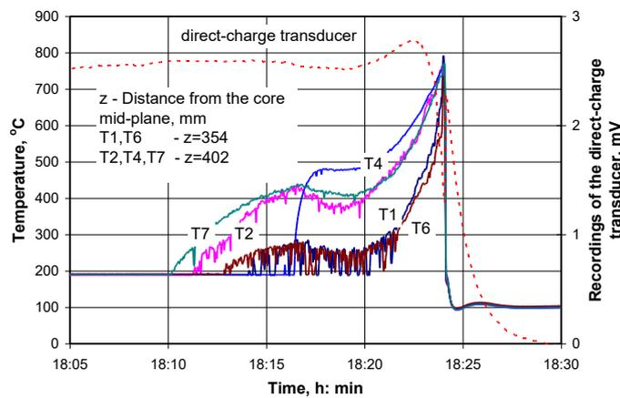
FIG. 6. Readings of the direct-charge detector. Data recorded by thermocouples attached on the claddings of fuel rodlets from the outer circle.
