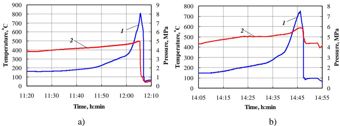
FIG.13. Cladding temperature variation with time (1) at 10 to 20 mm above the middle spacer grid and time history of gas pressure (2) in the lower gas plenum during tests 1 (a) and 2 (b)
