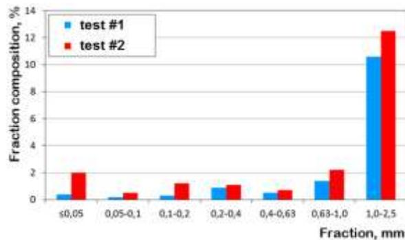
FIG.17. Grain particle size of extracted fuel.
