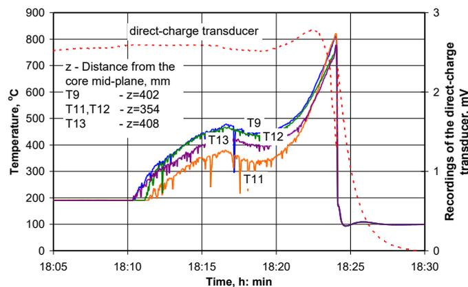
FIG. 7. Readings of the direct-charge detector. Data recorded by thermocouples attached on the claddings of fuel rodlets from the middle circle.
