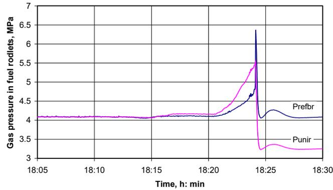
FIG. 8. Gas pressure in un-irradiated ( $P_{unir}$ ) and re-fabricated rodlets ( $P_{refbr}$ ).
