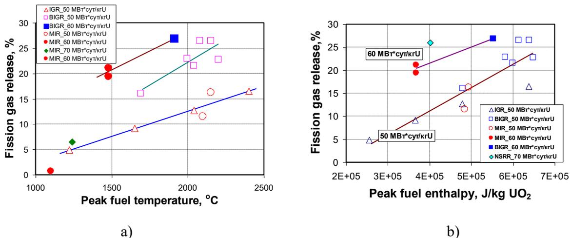
FIG.3. Fission gas release as a function of the peak temperature (a) and peak fuel enthalpy (b).
