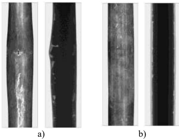
FIG. 14. Surface appearance of the cladding and X-ray images taken at place of cladding failure during test #1\* (a) and the maximum deformation during test #2(b)
