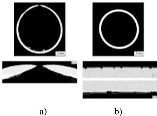
FIG.16. Fuel cladding structure after test #1 (a) at the rupture cross-section and after test #2 (b) at the cross-section of its maximum deformation.
