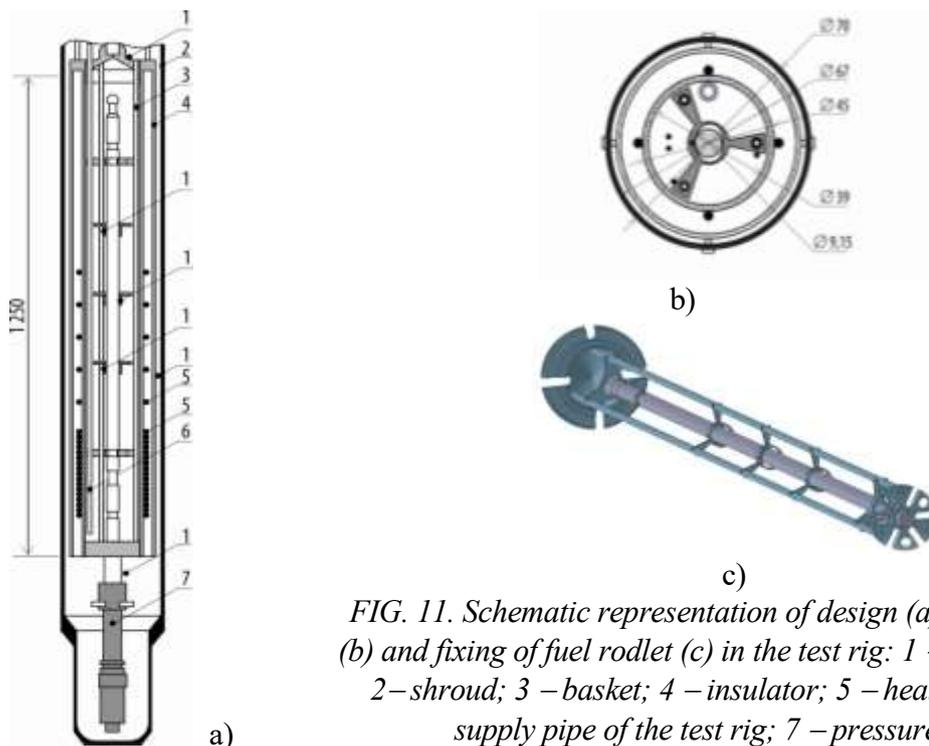
FIG. 11. Schematic representation of design (a), cross-section (b) and fixing of fuel rodlet (c) in the test rig: 1 – thermocouple; 2 – shroud; 3 – basket; 4 – insulator; 5 – heater; 6 – water supply pipe of the test rig; 7 – pressure gage.
