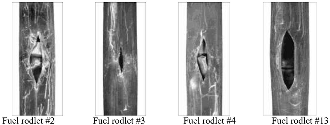
FIG. 9. Outer appearance of the claddings at the place of fuel failure.
