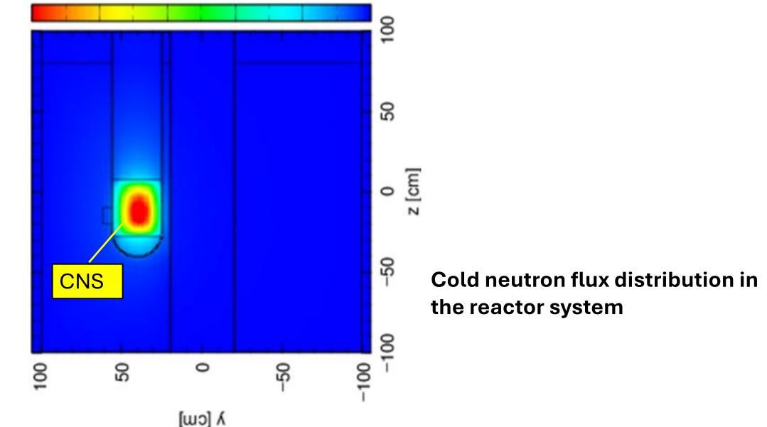
To extract cold neutrons from the center of the CNS, it is important to introduce a re-entrant structure—a shallow cavity on the CNS surface.
