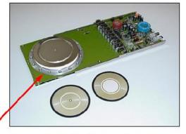
Reverse Conducting Discharge Device
