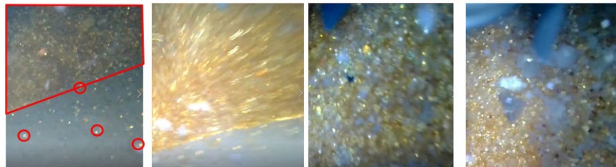
Observations of the resin in the storage tank. Fluidity was maintained.
