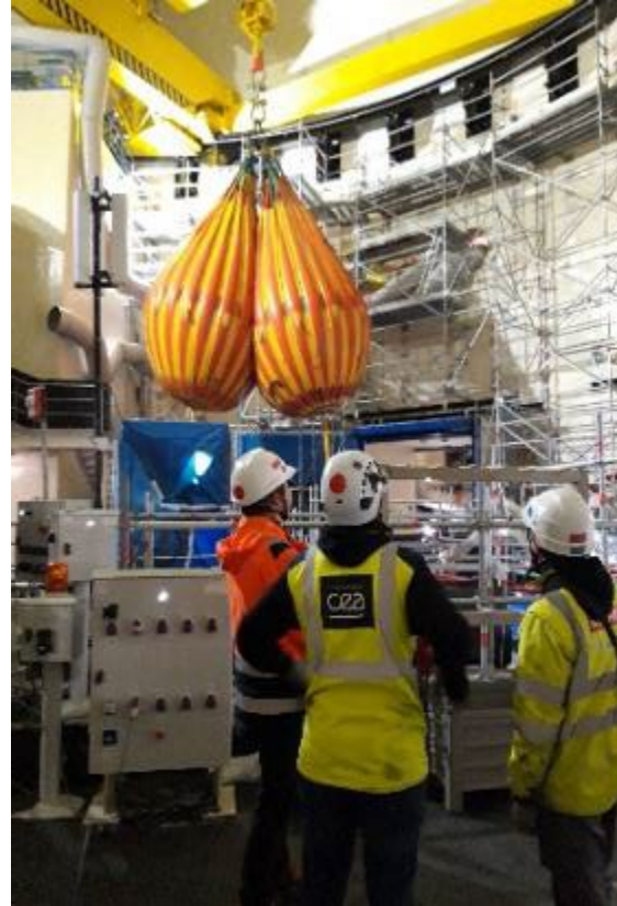
Polar Crane re-qualification in the Nuclear Reactor Building
