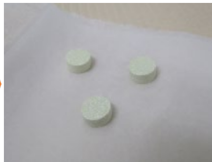
Pellet size: \phi 10 \times 5 mm Mass : 1.2 g Theoretical density: 70% Solubility: Dissolved in \text{NaOH}
